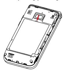
**Step 3.** To insert SIM card 1 or microSD card 2, push the SIM card or microSD card into the card slot with the gold-colored contacts facing down.
