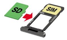
**NOTE:** If you need to install or reinstall your SIM card, remove the original SIM card from the tray and place your new SIM card into the tray with the gold contacts facing down as shown.
