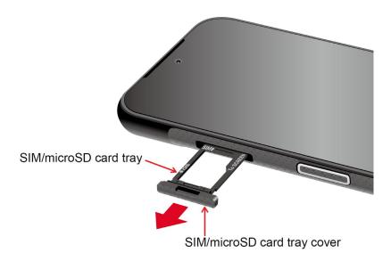
2. Put the tray onto a flat surface and place a microSD card into the tray. Ensure the gold contacts are facing down as shown.
