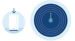
When the status LED is green, you are connected to the 5G or 4G network. The 5G LED will iluminate if a 5G network is found. Next three LEDs are indicating the signal strength.
