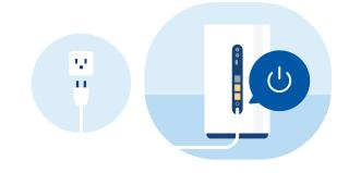
Plug in the power adaptor and then connect it to your gateway. Push the on/off button, the LEDs on the top of the gateway will turn on.
