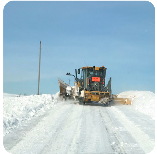
A Dubuque County motor grader, equipped with a front plow and wing blade, easily clears a gravel road.
